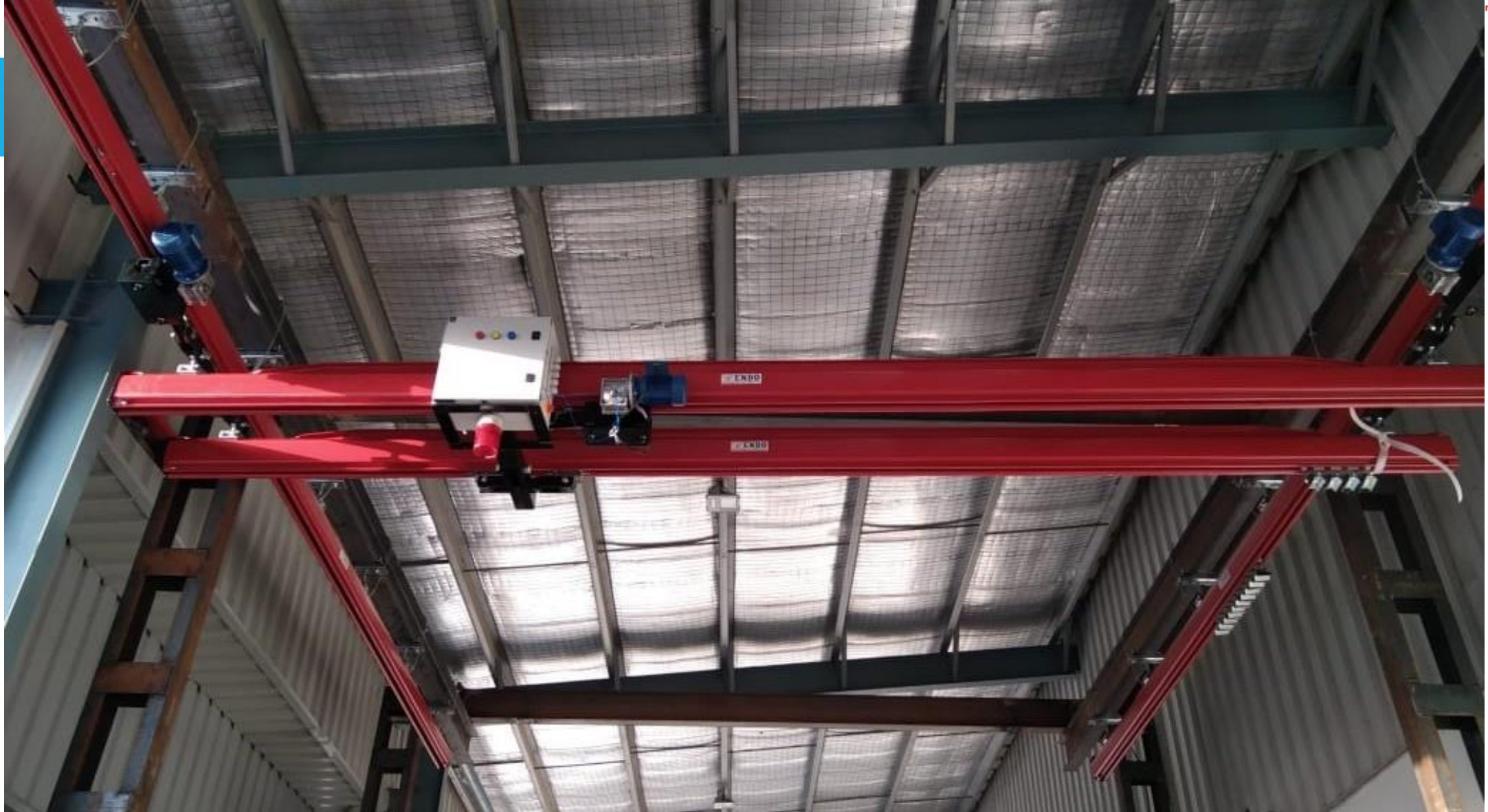
MOTORIZED XY RAIL SYSTEM 1.5T SWL
